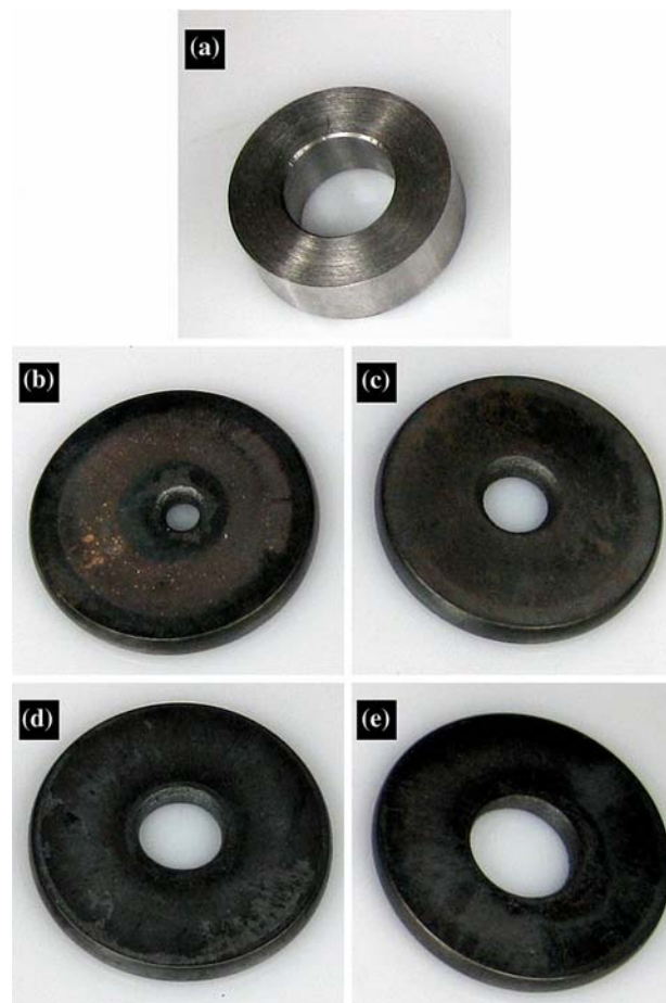
Fig. 11 Representative ring specimens before and after ring upsetting tests shown in the order: a before test, b without lubricant, c with NC-DEG, d with CMK-3, and e with reference lubricant
